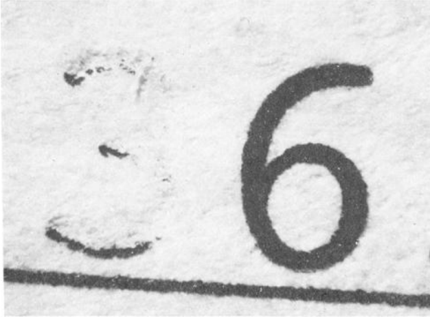
FIG. 1—Ink traces resulting from imperfect realignment of material in typewriter or “setting up” of ink on the paper.
